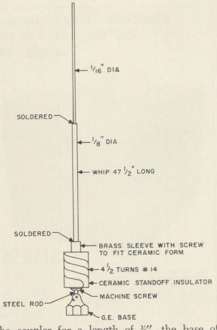
the coupler for a length of 4", the base of the whip is inserted from the opposite end and the three are then soldered together to make a rigid unit. Care should be taken to keep the solder off the threads of the machine screw.
